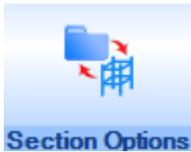
The section option allows the user to copy the selected set of rebar to an object. Rebar sections for footing, beam, column, etc. are available as inbuilt sections. A section can be added, renamed and deleted.
