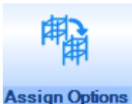
This option allows the user to assign the properties of one bar to another. Assign option allows the user to choose the bars from which the properties are to be assigned. Apply to screen option allows the user to choose the type of bar to which the property is to be applied to. The properties from the source bar can be applied to the entire set of bars or to the single run bar or to a single bar.
