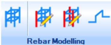
Rebar modelling allows the user to draw and edit the rebars in a concrete model. Rebars can be drawn using various draw options.
