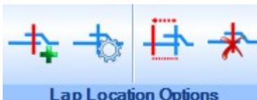
Lap location option allows the user to create locations for the bars to be lapped, to edit lap properties, to modify a lap location and edit the lap location.
